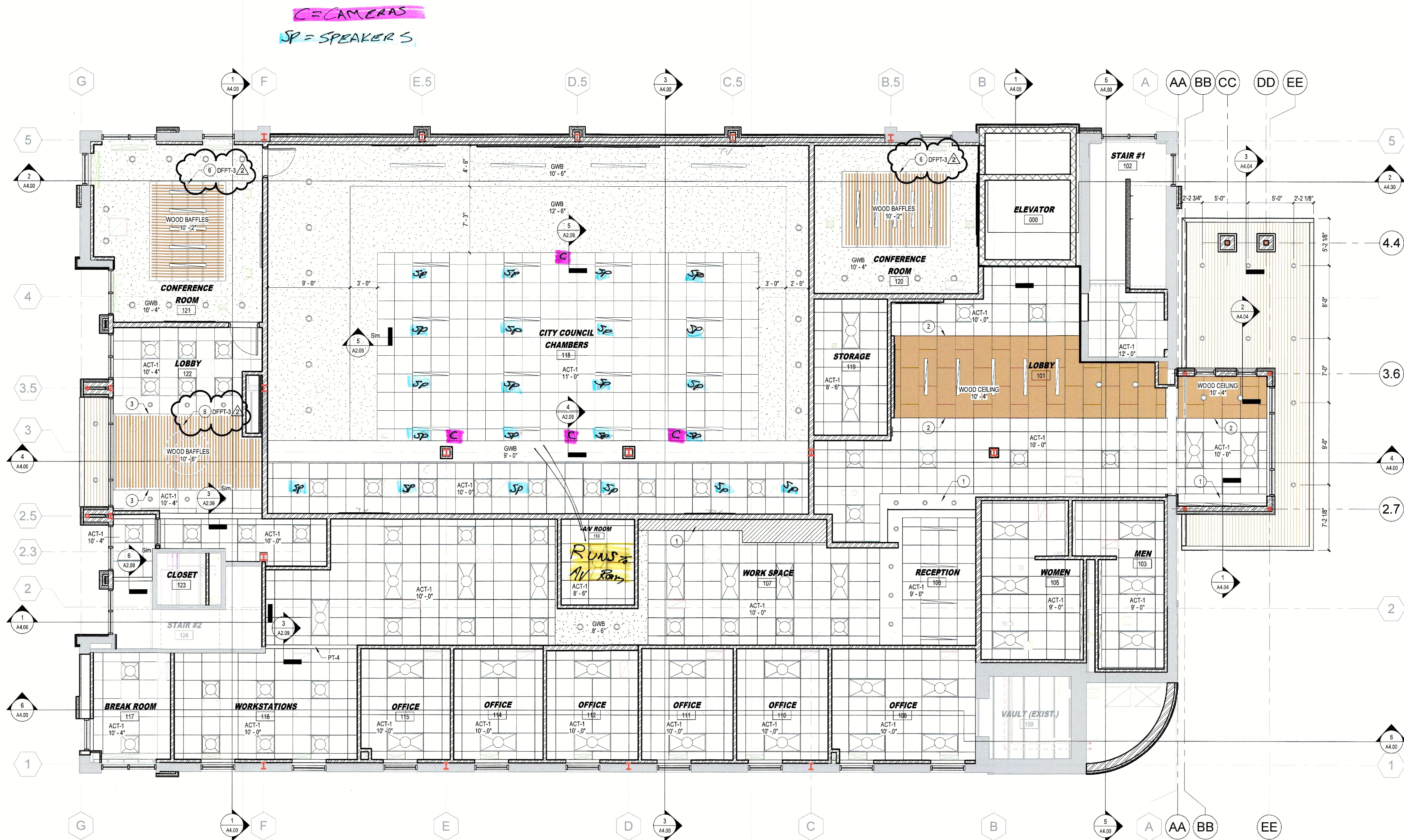
FLOOR 01 - REFLECTED CEILING PLAN 3/16" = 1'-0"
